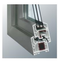
THERMAL TRANSMISSION: Uw to **0,76 W/m²K** STRENGTHENERS: steel reinforcement
